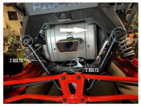
2. Remove the factory exhaust cover by removing the (2) Torx Bolts and remove towards the back of Vehicle. Next remove the (2) 13mm bolts on the bottom hanger exhaust bracket. This hanger will not be reused. Now remove the 8mm bolt holding the tip on and remove the tip. Now remove the factory muffler by removing the 2 14mm bolts securing the flange and slide the system to the passenger side to remove exhaust. (Inspect picture to pin point Bolt locations)
