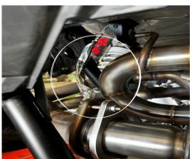
3. Remove Factory Gasket and re-install backwards. (you will simply flip the gasket from its original position.
