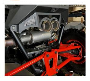
4. Next install the Gibson Beauty Plate #B using the 2 Factory Torx Bolts. With everything installed and now tight be sure to double check clearance of O2 wire and all other parts. We need a minimum of 1" of clearance. It is important that all parts are cleaned of grease, finger prints, and any sport of liquid to prevent staining. 304 is stainless not stainless. Re connect the battery cable and enjoy your new Gibson exhaust.
